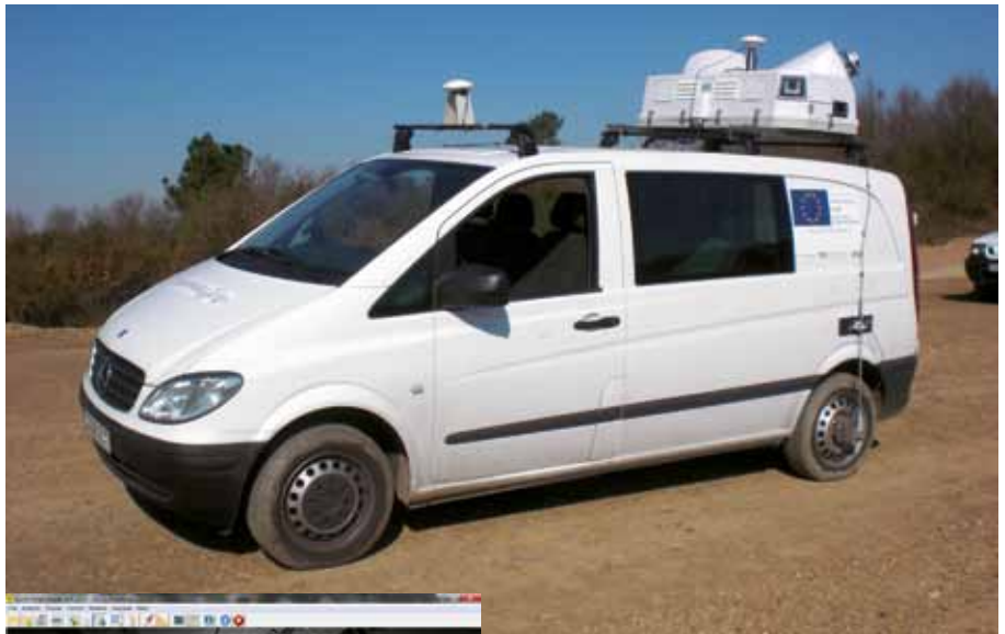
SITEGI is a mobile road infrastructure surveying system developed by the University of Vigo
